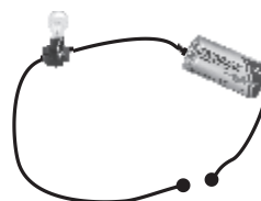
Open electric circuit
